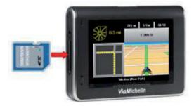
To remove the SD card from the device, press on the side of the SD card and release. The SD card will then be ejected from the device.
